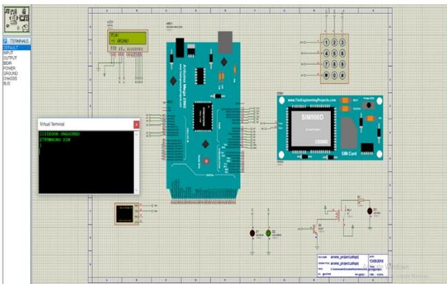
Fig 8: Simulation result for system response with the wrong password
