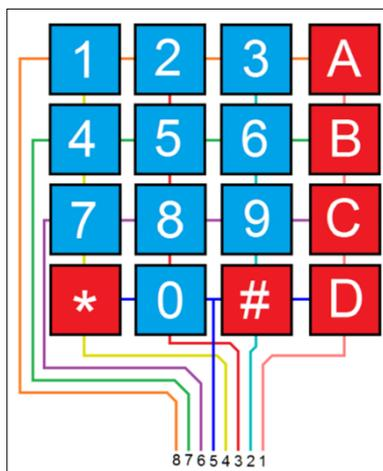
**Fig 3:** Matrix Keypad Connections
