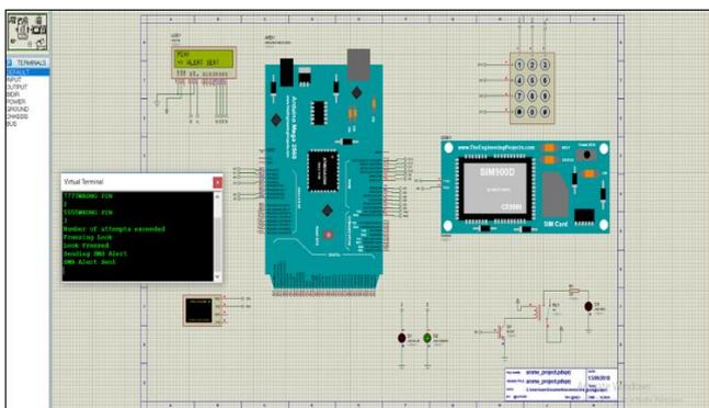
Fig 9: Simulation result for maximum attempts exceeded, lock frozen and sending alert
