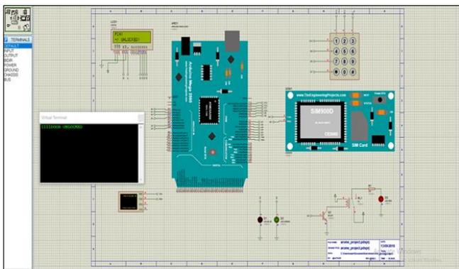
Fig 7: Simulation result for system unlocked using the right password
