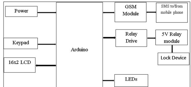
Fig 1: General block diagram for the system
