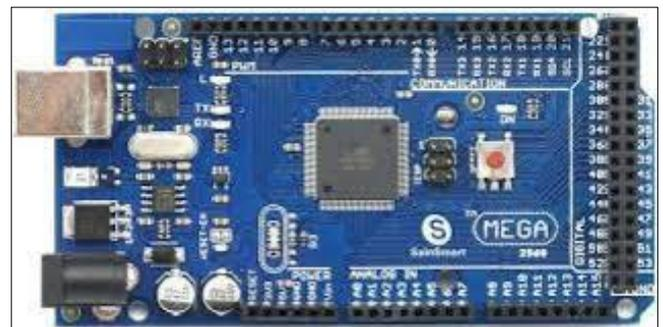
Fig 2: Arduino board with Atmega 2560.
