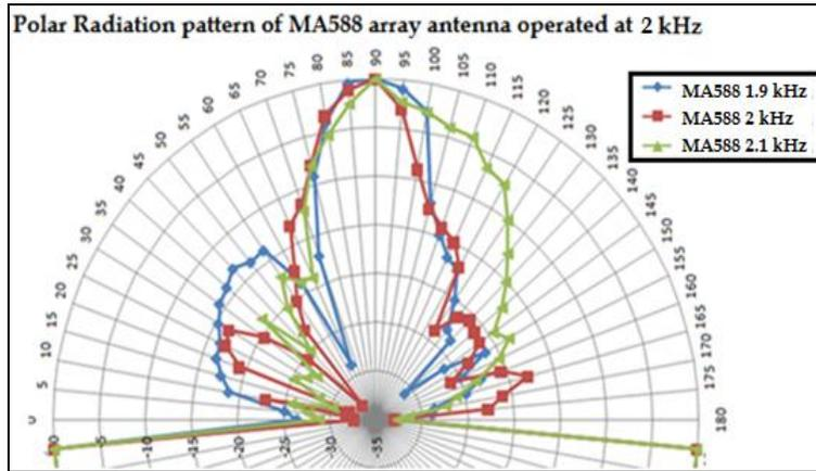
**Fig 7:** Normalized polar Radiation pattern of the uniform  $8 \times 8$  MA588 array antenna at three frequency steps 1.9 kHz, 2 kHz, 2.1 kHz.
