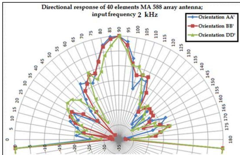
**Fig 9:** Directional response of MA588 array antenna of 40 elements
