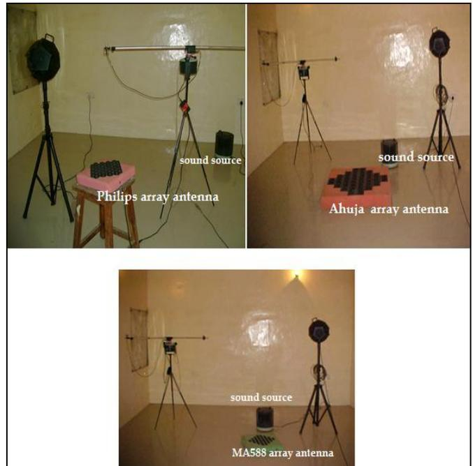
**Fig 4:** Experimental set-up in reverberation chamber for three different radiators array antenna
