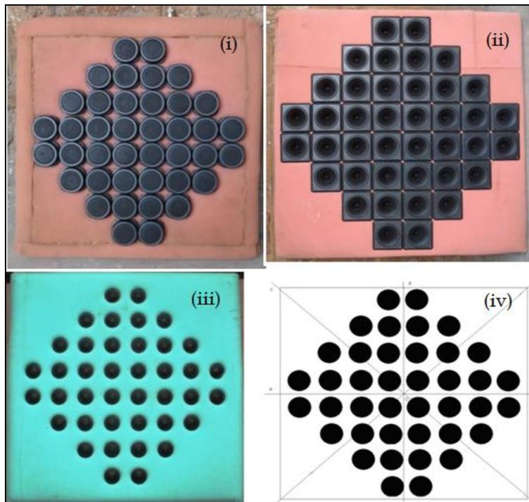
**Fig 1:** Photograph of the array antenna made 40 elements (i) Philips (ii) Ahuja (iii) MA588 tweeters and (iv) tweeters outlay
