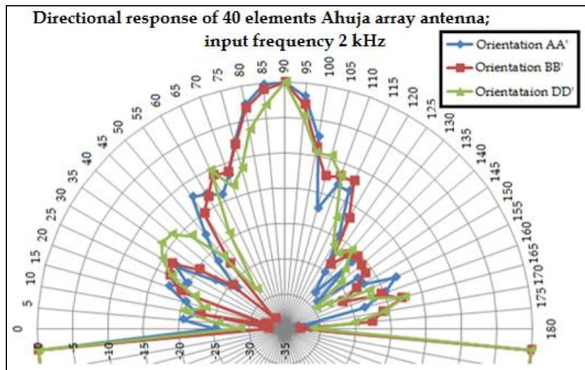
**Fig 10:** Directional response of Ahuja array antenna of 40 elements
