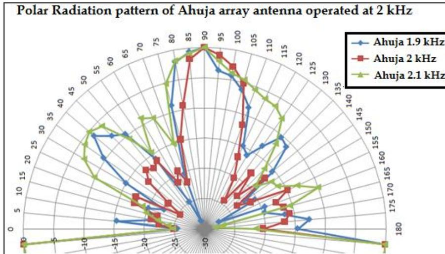
Fig 5: Normalized polar radiation pattern of the uniform 8 x 8 Ahuja array antenna at three frequency steps 1.9 kHz, 2 kHz and 2.1 kHz.
