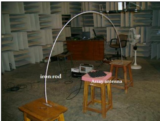
**Fig 3:** The experimental setup of Philips array antenna in the anechoic chamber
