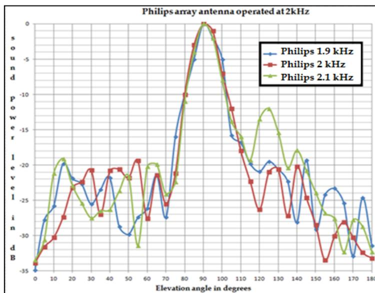
Fig 6: Normalized Radiation pattern of the uniform 8 x 8 Philips array antenna at three frequency steps 1.9 kHz, 2 kHz, 2.1 kHz.
