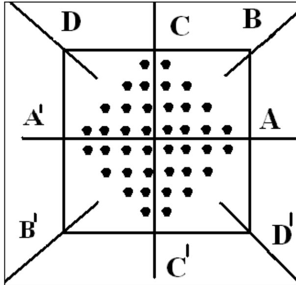
**Fig 8:** Directional response of the antenna with 40 radiators in three different orientations
