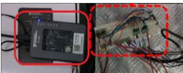
Fig 10: DAQ module and input-output circuit
