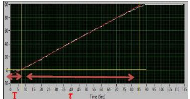
Fig 15: Acquiring dead time and compensating time values using ZN open loop test.
