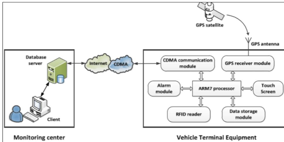
**Fig 7:** Block diagram of GPS tracking system
