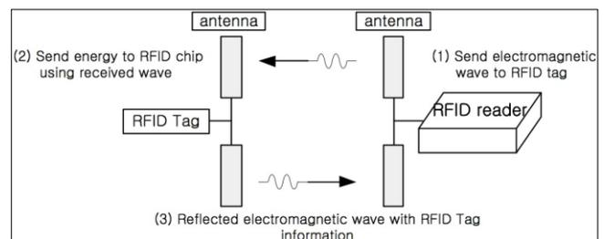
Fig 1: RFID block diagram
