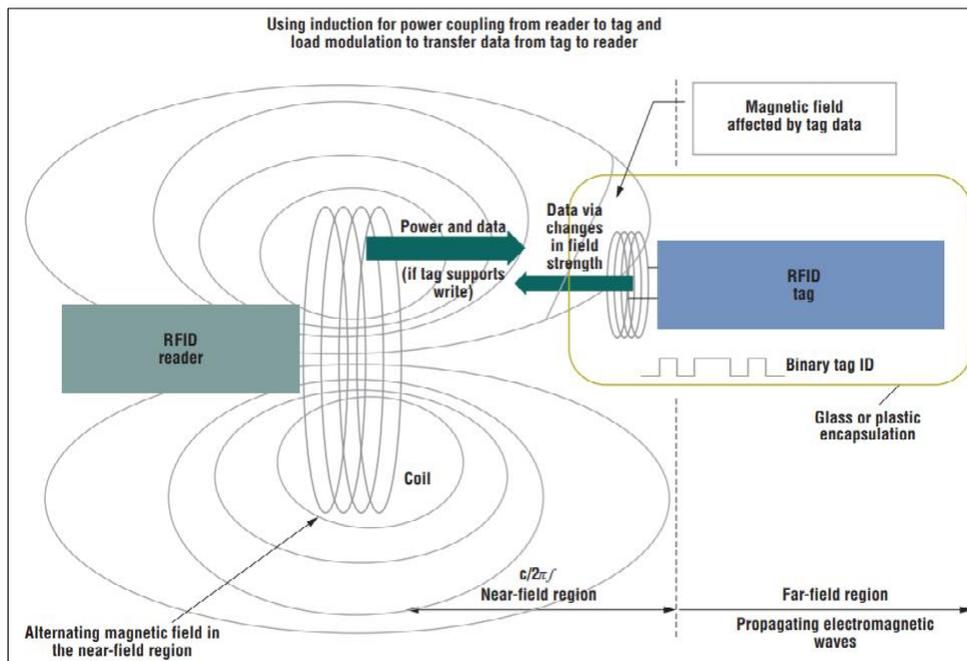
Fig 2: Near-field power/communication mechanism for RFID tags operating at less than 100 MHz
