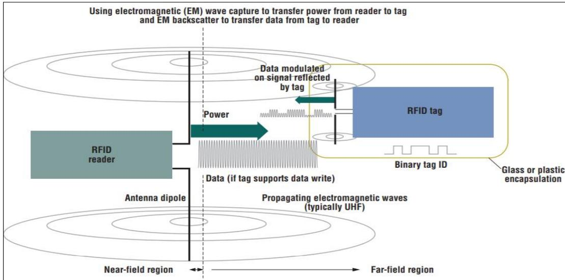
Fig 3: Far-field power/communication mechanism for RFID tags operating at greater than 100 MHz
