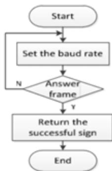
Fig 4: Initialization of RFID reader
