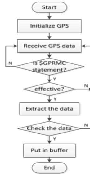
**Fig 6:** Extracting the location data by GPS
