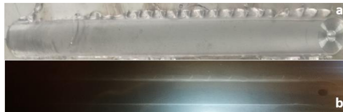
Fig 3: Photographs shows (a) general appearance and (b) X-Ray Radiography of joints FS welded using 1400 rpm and 100 mm/min.
