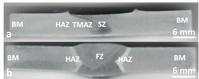
Fig 5: Macrographs of the joints welded using; (a) FSW at 1120 rpm and 100 mm/min; and (b) GTAW at 175 A and 17 V.
