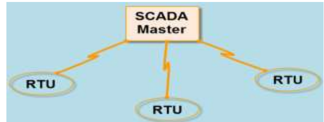
Fig 1: Network architecture of Monolithic or Early SCADA Systems [8]
