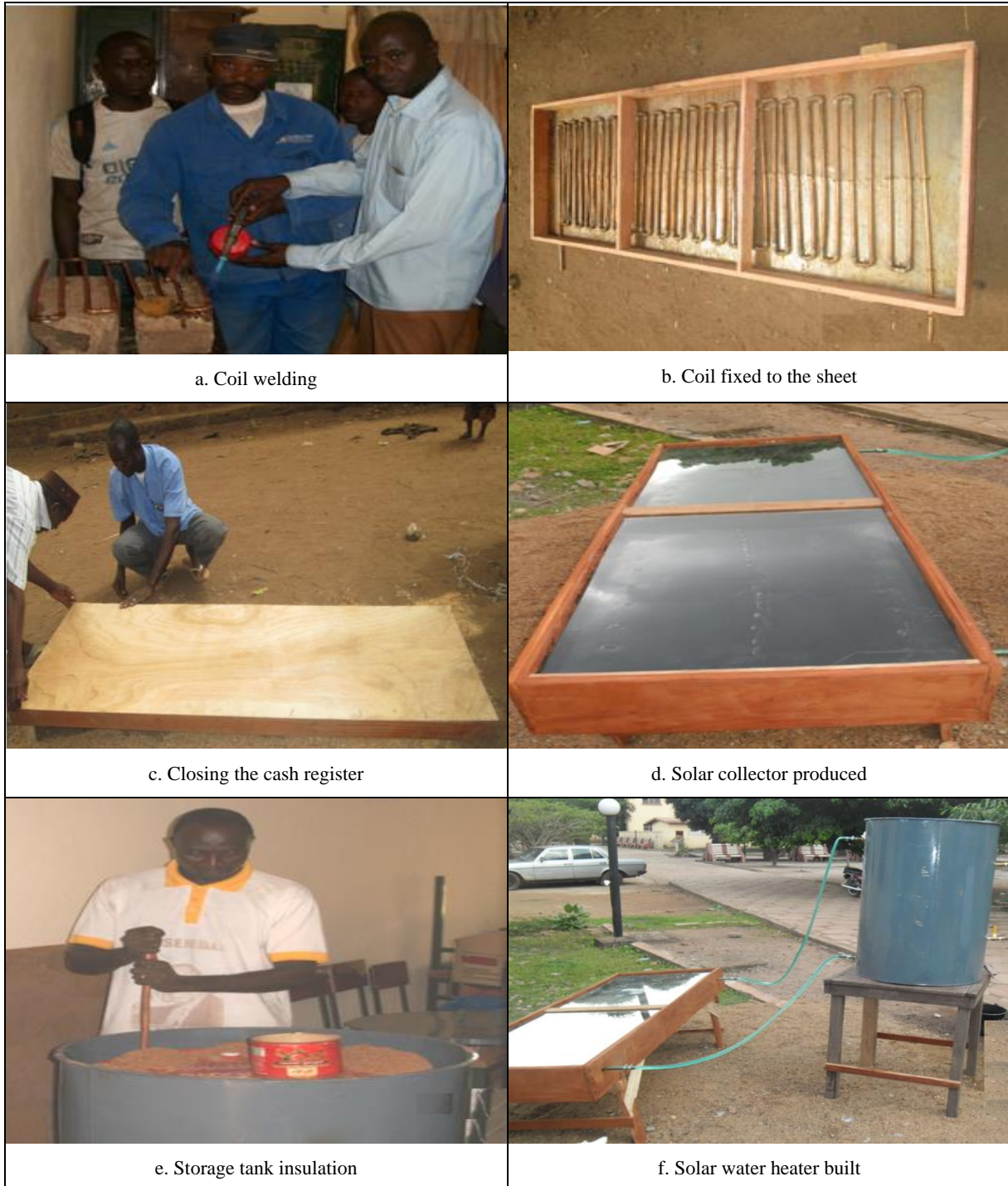
Fig 1: Steps in building the solar collector
