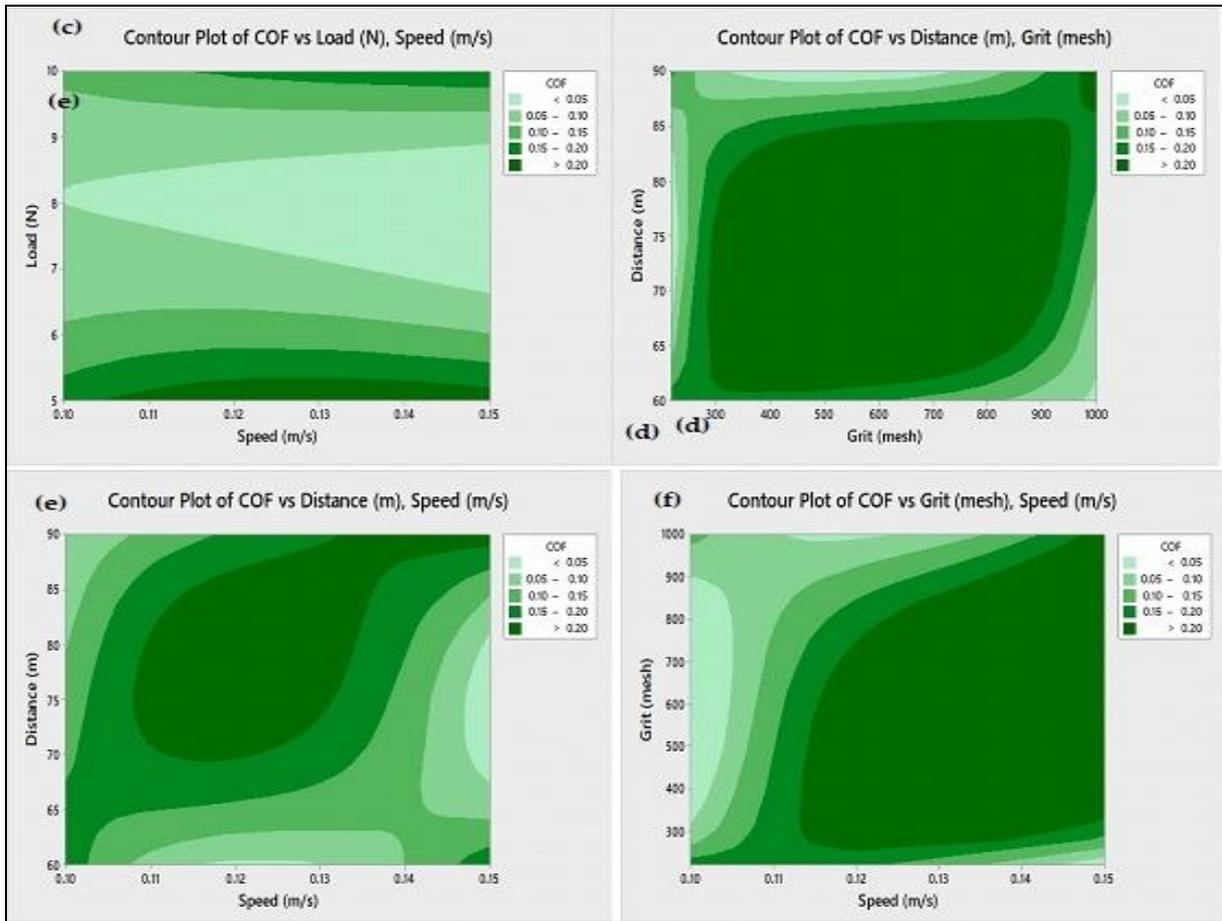
Fig 4: Contour plots for COF (a) L vs. D (b) L vs. G (c) L vs. S (d) D vs. G (e) D vs. S (f) G vs. S
