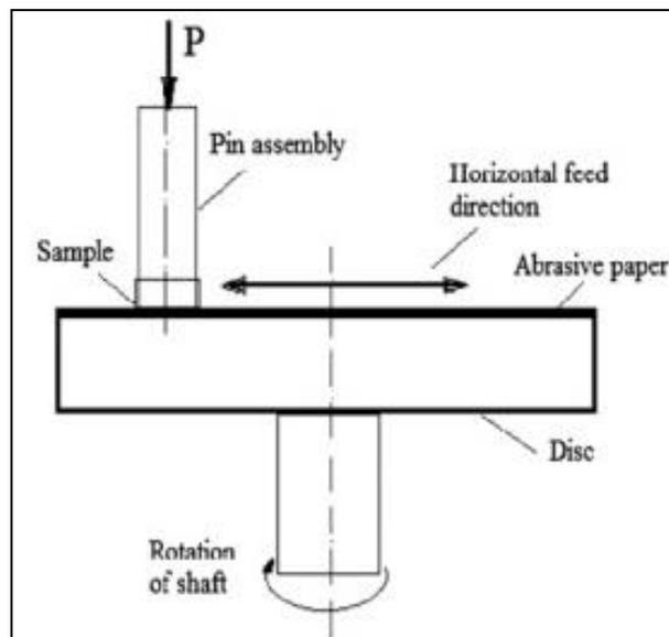
**Fig 1:** Schematic view of a pin-on-disc kind of arrangement
