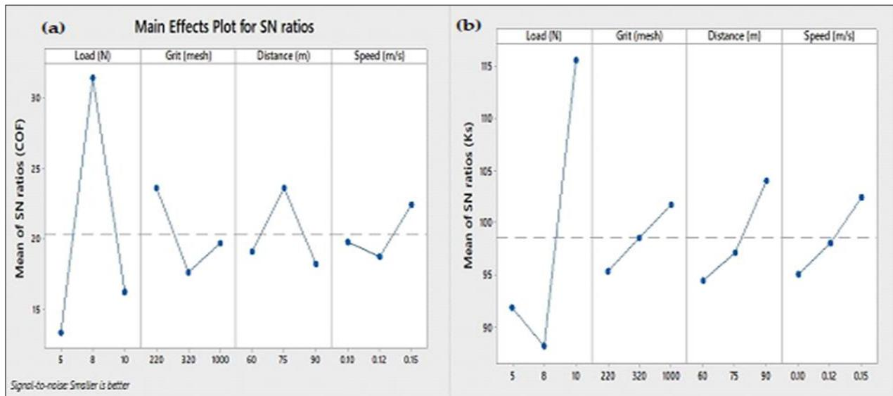
Fig 3: Main effects plot for (a) COF and (b) Ks
