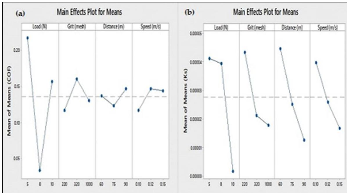
Fig 2: Effect of process variables on (a) COF and (b) Ks
