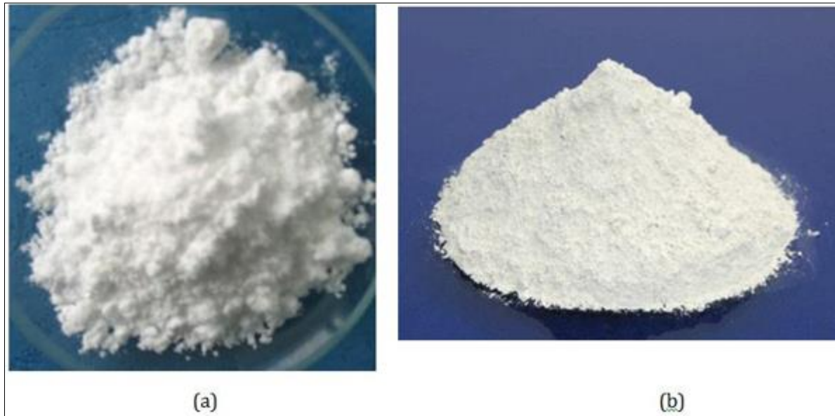
Fig 1: Modifiers of asphalt binder (a) Al 2 O 3 nano particles (b) CaCO 3 nano particles.
