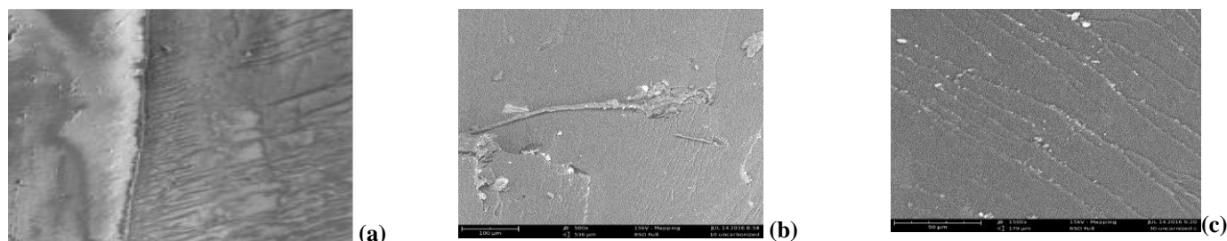
Fig 4: SEM Micrograph of reinforced polyester composite. (a) Unreinforced polyester resin (b) 10% uncarbonized fine coconut shell particles (c) 30wt. % uncarbonized coarse coconut shell particle. International Journal of Research in Advanced Engineering and Technology
