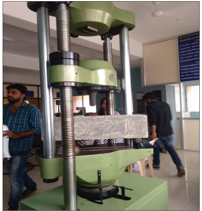
Fig 10: Placing of Beam in UTM Machine
