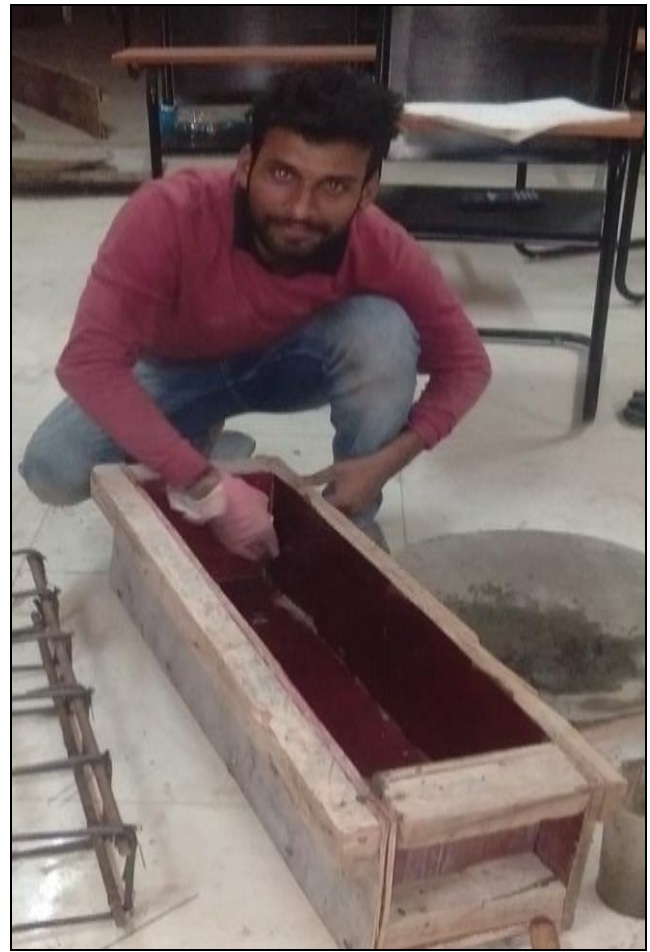
Fig 5: Formwork of Beam mould
